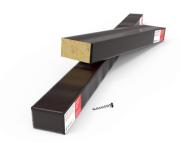
Tenmat's VFB 120/120 Ventilated Fire Barriers are 'open state' cavity fire barriers for ventilated cavities of up to 450mm. Each VFB 120/120 consists of a specially formulated fire rated stone mineral wool section with an integral high expansion intumescent seal fixed to the leading edge.
