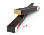
Tenmat's VFB 60/60 Ventilated Fire Barriers are 'open state' cavity fire barriers for ventilated cavities of up to 450mm. Each VFB 60/60 consists of a specially formulated fire rated stone mineral wool section with an integral high expansion intumescent seal fixed to the leading edge.
