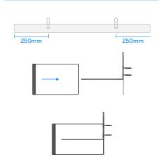
For cavity barriers 91mm-215mm wide (across cavity) use 2 MP brackets and the 160mm long spike. The 160mm spike will require cutting to size, if used in barriers less than 185mm wide, to ensure that the spike does not pierce through the face of the intumescing material, the bracket should be cut to provide a minimum projection through the barrier to 3/4 of the cavity barrier width and to a maximum of 25mm behind the face of the intumescing strip.
