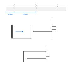
Fix 3 number MP brackets, per linear meter, to the substrate at maximum 150mm from the end of the cavity barrier, with a maximum spacing between brackets of 350mm.
