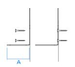
For cavity barriers 76mm-90mm wide (across cavity) use 2 MP brackets and the 65mm (A) long spike.
